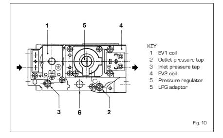
pressure regulator on the valve until the exact value is obtained. Screw slowly and gradually. Read the gas meter at least thirty seconds after regulating the pressure.
