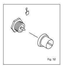
To start the boiler again, switch off the power, then remove the smoke stat cover and reset the button below (fig. 12).
