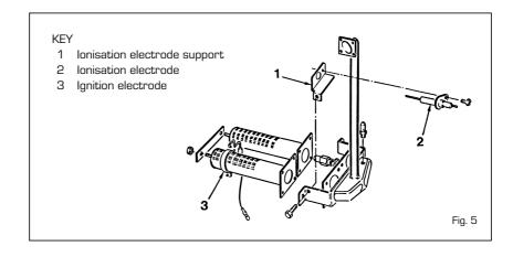
board; the lamp will light if there is power. At this stage the boiler will start to work sending, via the FM 11 programmer, a discharge current to the electrode and, at the same time, opening the gas valve. Normally the burner takes 1 or 2 seconds to light.
