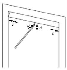
A.25mm down from top of opening B. 25mm in from front of opening. C. Disregard outer 50mm either side of fireplace opening
