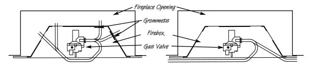
If using an across the hearth connection, the pipe work must be channelled through one of the cut outs in the ashpan.
