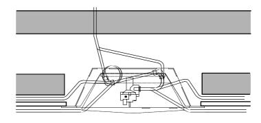
ing fixing. An isolator cock or restrictor elbow must be fitted to the incoming supply to facilitate servicing.
