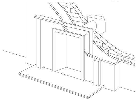
Where removal of any part of a timber frame is undertaken, the structural integrity of the wall must be retained. The advice of your local building control officer should be sought. If the property is under any NHBC warranty it is also advised that their advice on this kind of modification is sought.
