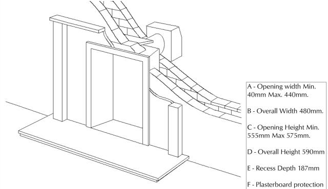
This method allows for installation of the appliance with the rear part recessed into the inner leaf of a cavity wall. This should enable a standard fire surround and back panel/hearth set to be fitted to the wall with the fire presented naturally in a flush fitted manner. The structural integrity of the wall must be maintained.
