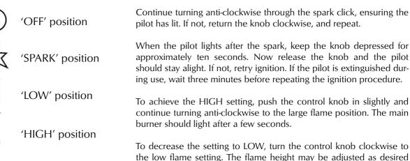
the low flame setting. The flame height may be adjusted as desired between high and low settings by turning the control knob to the HIGH' and 'LOW'. To turn to the PILOT position from the HIGH or LOW positions
