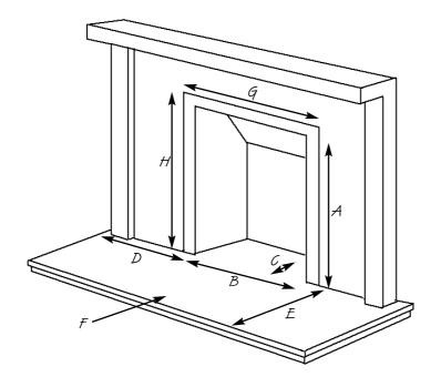
A. Opening height: 540mm min/575 mm max. B. Opening width: 365mm min/440mm max. C. Mounting depth: 285mm D. Hearth must extend minimum of 150mm either side of the opening. E. Hearth must extend minimum of 325mm in front of the opening. F. Non-combustible hearth must be a minimum of 50mm in height, or be surrounded by 50mm high fender. G. 470mm, this area must be flat and vertical to ensure a good seal. H. 585mm, this area must be flat and vertical to ensure a good seal.
