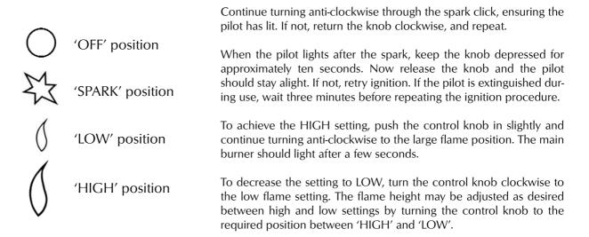
To turn to the PILOT position from the HIGH or LOW positions, press the control knob in, and return to the pilot position and release.
