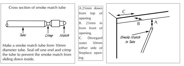
NOTE: If spillage is still indicated after undertaking all of the above, there may be a fault in the flue, or insufficient ventilation is present.
