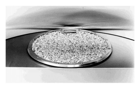
2. Place the ceramic log support centrally on top of the vermiculite bed as shown. The four flat faces of the log support should be facing downwards. Do not press the log support downwards, as this will compact the vermiculite.
