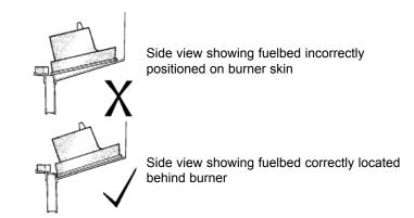
Position upper fuelbed component on to the locating pegs on the top of the fuelbed base, ensuring that it is correctly seated as shown below in fig. 12
