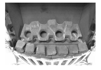
e) Select the four coals and arrange along the front of the fuelbed, directly behind the front row of coals. Leave gaps between the coals in line with the front flame notches on the front of the fuelbed (shown below arrowed), this enhances the front flames and provides the most pleasing flame effect. Select the two **smallest** coals and place them at each end of the second row of coals. See fig. 15 below.
