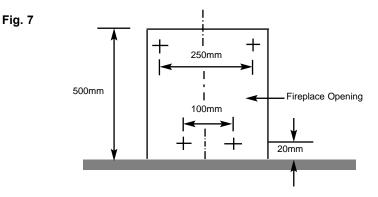
Fit the wallplugs provided and screw the fixing eyes securely into the rear of the fire opening. If the clearance at the rear of the fire is at the minimum specified for a precast flue application, it may be necessary to bend over the lower fixing eyes after screwing them fully in to the rear of a pre-cast starter block.
