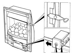
Unscrew the burner assembly fixing screws at either side of the firebox, and the two fixing screws at the base of the fire (See fig. 7 below). Carefully pull the base of the burner forwards from the fuel-bed support panel. The burner can now be removed from the appliance.
