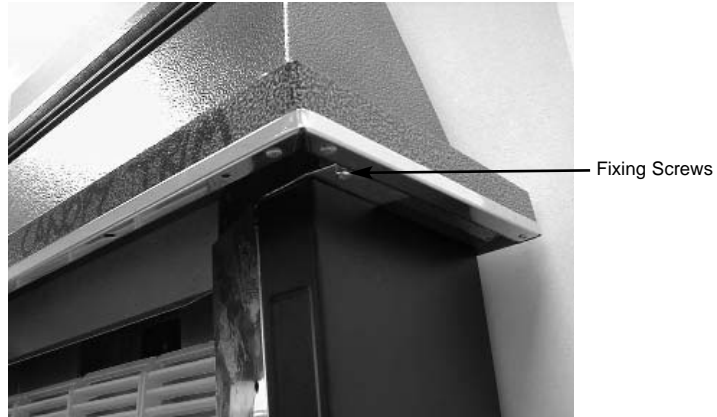
Fig. 6 Removing the Upper Outer Case Fixing Screws
