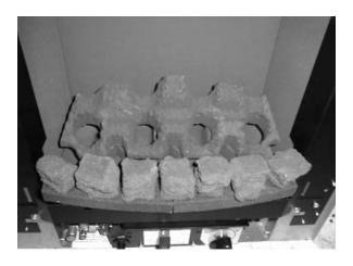
e) Select the four coals and arrange along the front of the fuelbed, direct ly behind the front row of coals. Leave gaps between the coals in line with the front flame notches on the front of the fuelbed (shown below arrowed), this enhances the front flames and provides the most pleasing flame effect. Select the two **smallest** coals and place them at each end of the second row of coals. See fig. 14 below.
