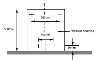
Fit the wallplugs provided and screw the fixing eyes securely into the rear of the fire opening. If the clearance at the rear of the fire is at the minimum specified for a precast flue application, it may be necessary to bend over the lower fixing eyes after screwing them fully in to the rear of a pre-cast starter block.
