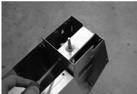
Fig. 12 Control Valve Panel Removal
