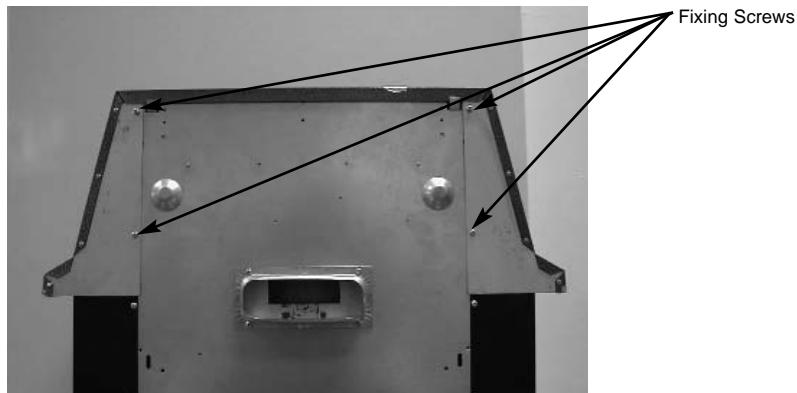
Fig. 7 Removing the four canopy rear fixing screws
