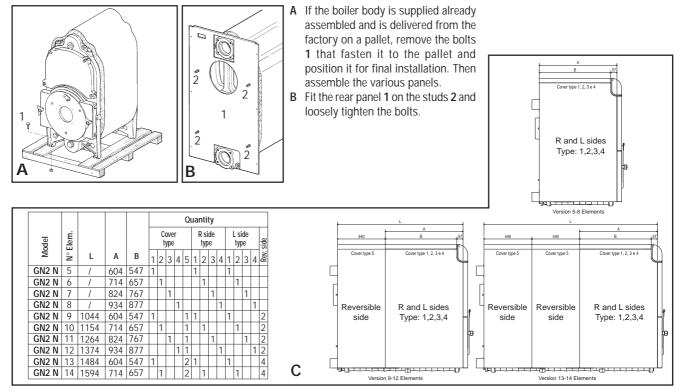
C Prepare the right and left sides, choosing the quantity of side panels according to the dimensions of the boiler (see table).
