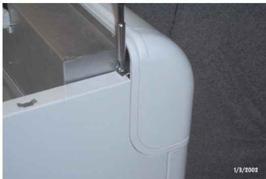
Fig. 5 - Unscrew and take out the two screws and both plates holding the control panel.
