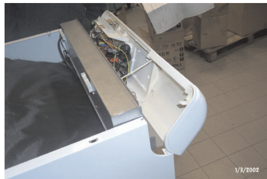
Fig. 6 - Turn the control panel forwards.
