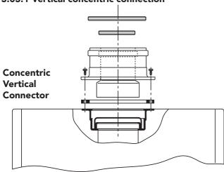
A vertical connector can be supplied for vertical discharge with concentric pipes.
