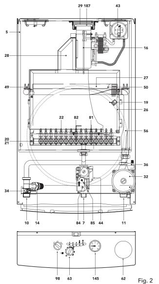
2.03 Boiler water flow diagram
