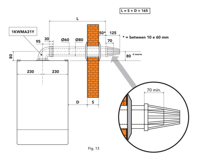
Slope downwards away from the boiler at a rate of about 3 mm/m to avoid rainwater entering the boiler.
