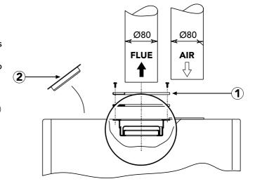
Connect flue duct to central hole Ø80 and air duct to left or right air intake hole Ø80. Insert blanking plate (2) in remaining air intake.
