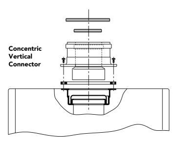
A vertical connector can be supplied for vertical discharge with concentric pipes.
