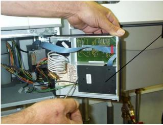
Locate the standard interface, bottom R/H corner in the R/H door
