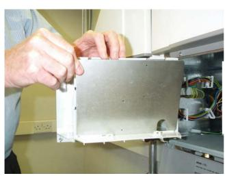
Gently prise back the 4 plastic retaining clips and remove the steel closing plate from the back of the left hand door.
