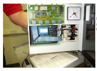
Re-connect data cable to *rematic*® interface and close smoked grey panel. And re-fit the PCB back into the L/H corner
