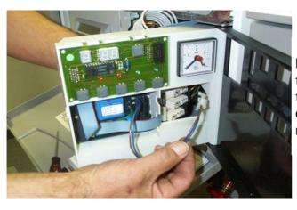
Fit new *rematic*® interface making sure that the blue/brown cables & connector board pass through slot by the PCB and the green/black cable passes through the slot in the Interface recess.
