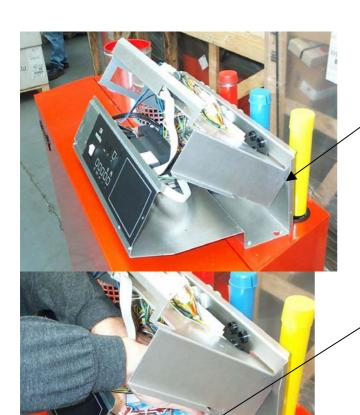
Raise and tilt the terminal strip assembly locking it onto the slots on the rear support as shown in picture
