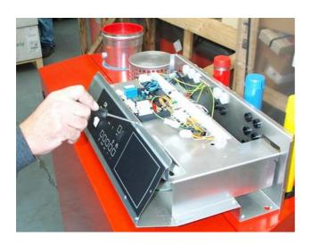
Release the front panel screws
