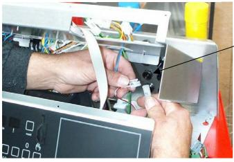
Find plugs K1 and K2 in the control panel wiring and fit the matching K1 and K2 plugs on the adapter plate harness
