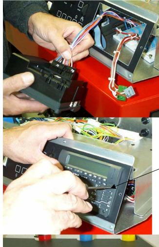
Take the remaining 4 plug units on the adapter plate harness and feed through the opening. Insert the plugs (two black, one green and one grey) into positions P3,P2,P11 and P12 in the back of the *rematic*® 2945 C3 K control unit
