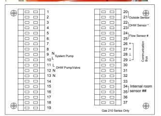
Mount the outside sensor in a sheltered position on a north facing wall - wire back to boiler (max 100M) Fit flow sensor (only required for multiple boilers) on the common flow pipework
