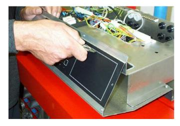
Lower terminal assembly back into place and secure
