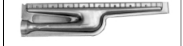
Figure 10 - Individual Burner Removed from the Burner Rack
