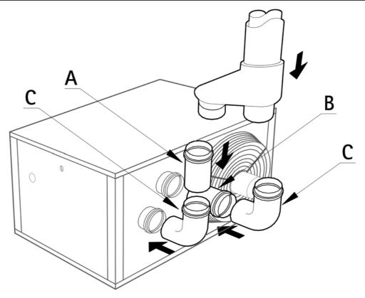
SCA/C4000S Vertical Transition Kit comprises on 2 off 90° elbows and 2 off short sections of pipe cut to length as per the following table:
