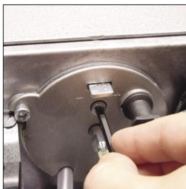
fig. 15 : Combustion head adjuster screw
