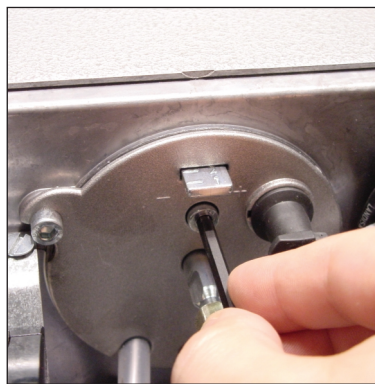
Fig. 12: Combustion head adjustment screw
